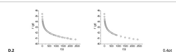
**Left**: F(t) sampled at unequal time intervals. **Right**: F(t) sampled at equal time intervals for  $t>1000~{\rm s}$ .
