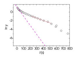
The best straight line in the range 200-500 s yield the parameters  $\tau_2$  and  $E_2$  (Question D.11). The slope of the best straight line in the range [10,30] s give an estimate of  $\tau_3$  (Questions D.12 and D.13).
