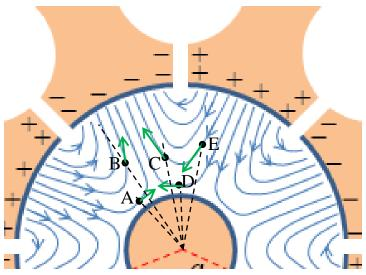
pointing clockwise therefore the electrons there drift towards the cathode, while for points C, D and E the azimuthal component points counterclockwise and the electrons there drift toward the anode.
