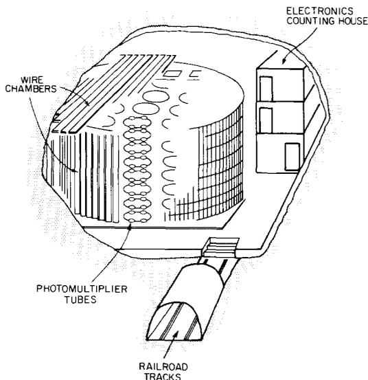
Fig. 1. Schematic representation of the HPW detector, showing the physical construction of the detector.
