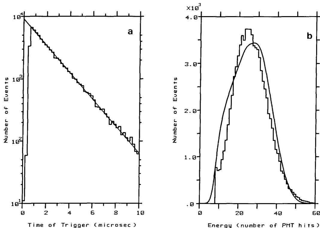
Fig. 3. Characteristics of secondary triggers with muon decays. (a) shows the time of the trigger, along with the predicted exponential lifetime based on the lifetimes of positive and negative muons in water and the measured charge ratio [6]. (b) shows the measured energy distribution of the muon decay triggers along with the Monte Carlo prediction in units of photomultiplier (PMT) hits.
