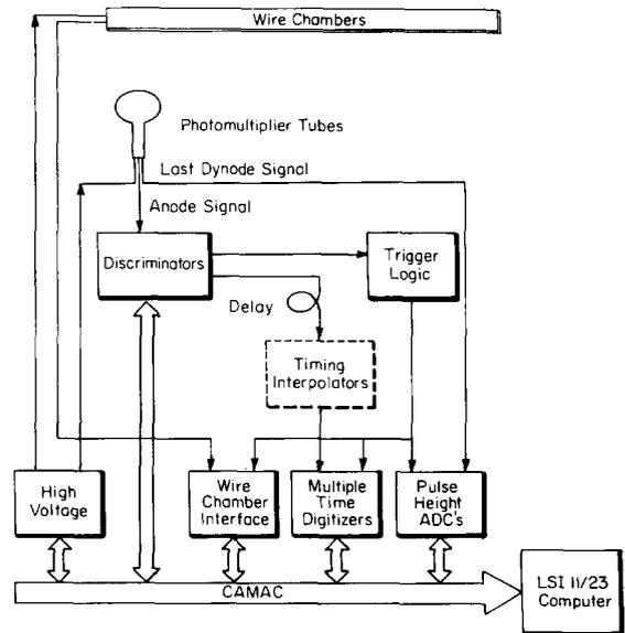
Fig. 2. Schematic representation of the data acquisition electronics. The timing interpolators were added half way through the data set and improved the time resolution from 8 ns to 3 ns.
