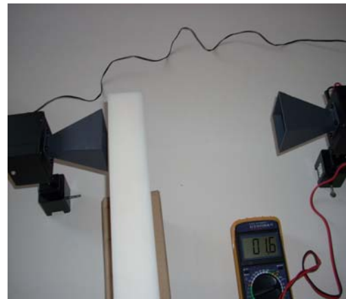
Figure 2. Microwaves pass through the dielectric.
