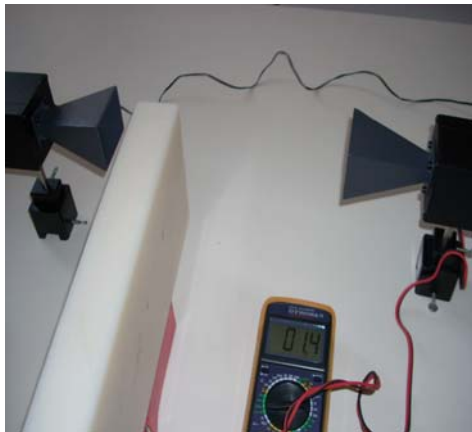
Figure 1. Half microwaves pass through the dielectric.
