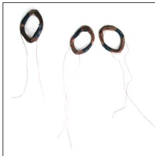
Figure 1 – Constructing the coils for the first device
