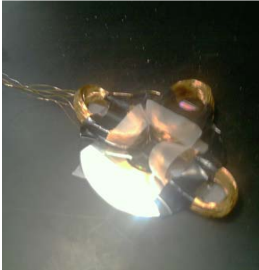
Figure 2 – Building the stator
